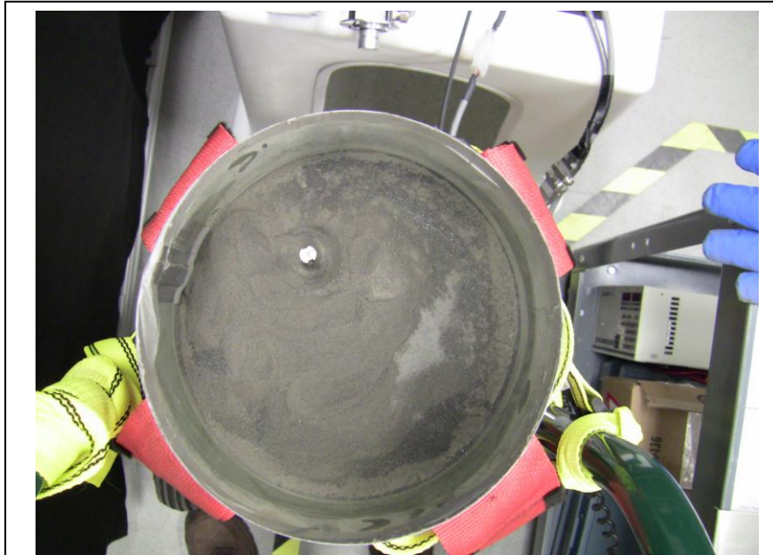
Figure 12. Top surface of 1-meter column with embedded penetrometer rod.
