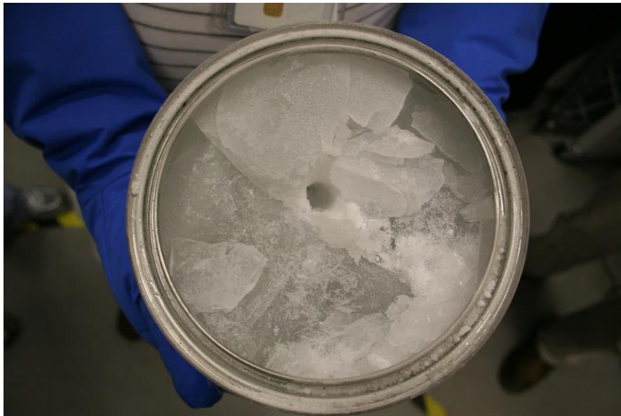
Figure 10. Fractured surface of can #5 with 100% water ice.
