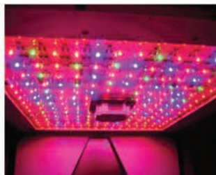
Veggie LED light bank.
