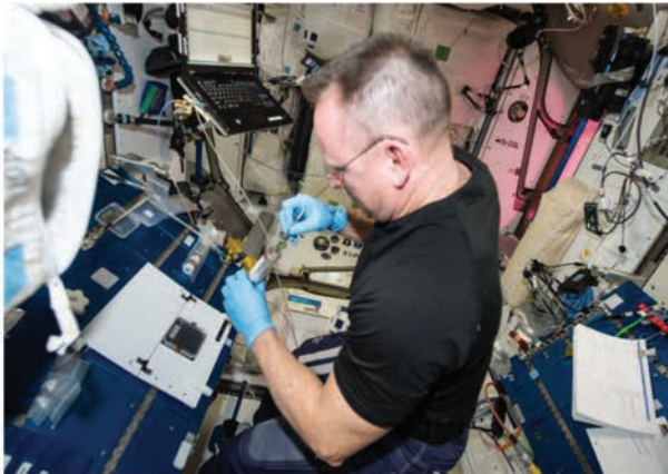
Astronaut Butch Wilmore fixing plants on the ISS using a Kennedy Space Center Fixation Tube (KFT) .
