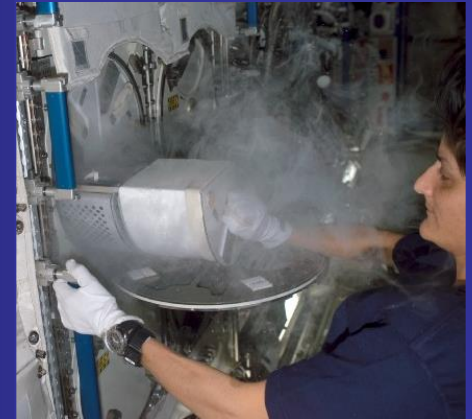
Sunita Williams inserting blood samples into the Minus Eighty Degree Laboratory Freezer
