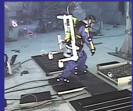
Example of a study on the effects of center of gravity on performance
