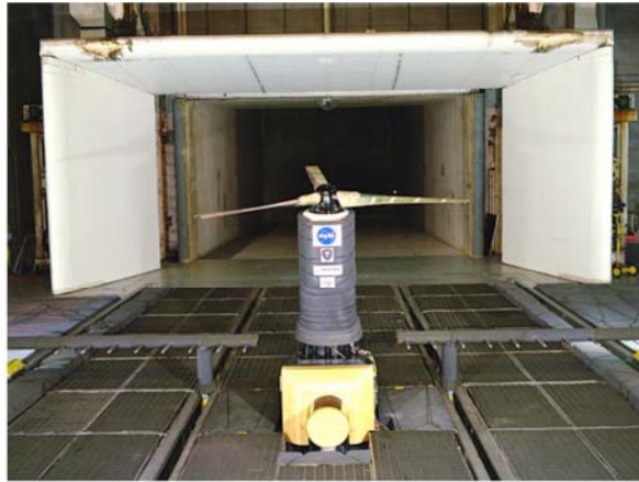
Figure 1. Rotorcraft model, traversable acoustic rake, and treatments in the 14x22 tunnel during a 1998 entry.
