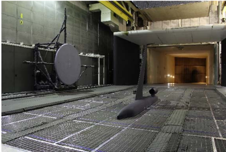
Figure 4. Sideline configuration of phased array, looking at pressure side of semi-span model.
