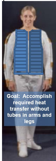
Figure 3. The high performance LCVG concept provides all of the required cooling in the torso region of the body
