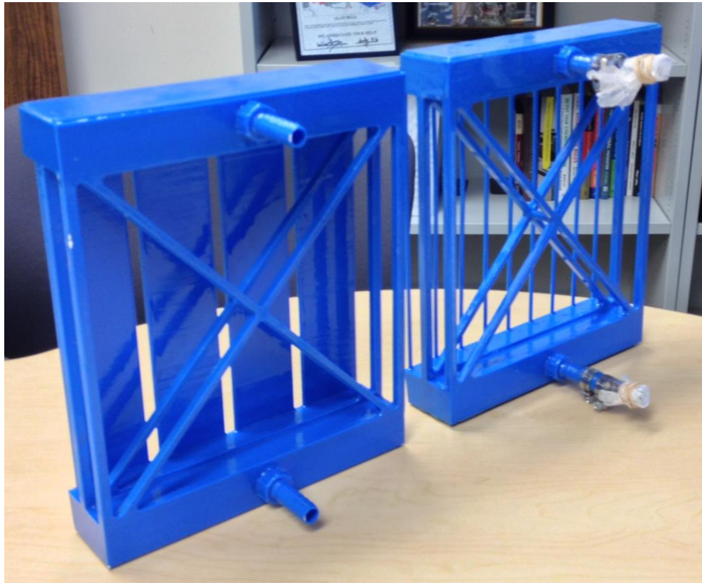
Figure 11. Test article surface that would sit on the hot plate is facing away from the reader in this view and the barbed fittings representing the inlet and outlet ports of the test articles are facing the reader.
