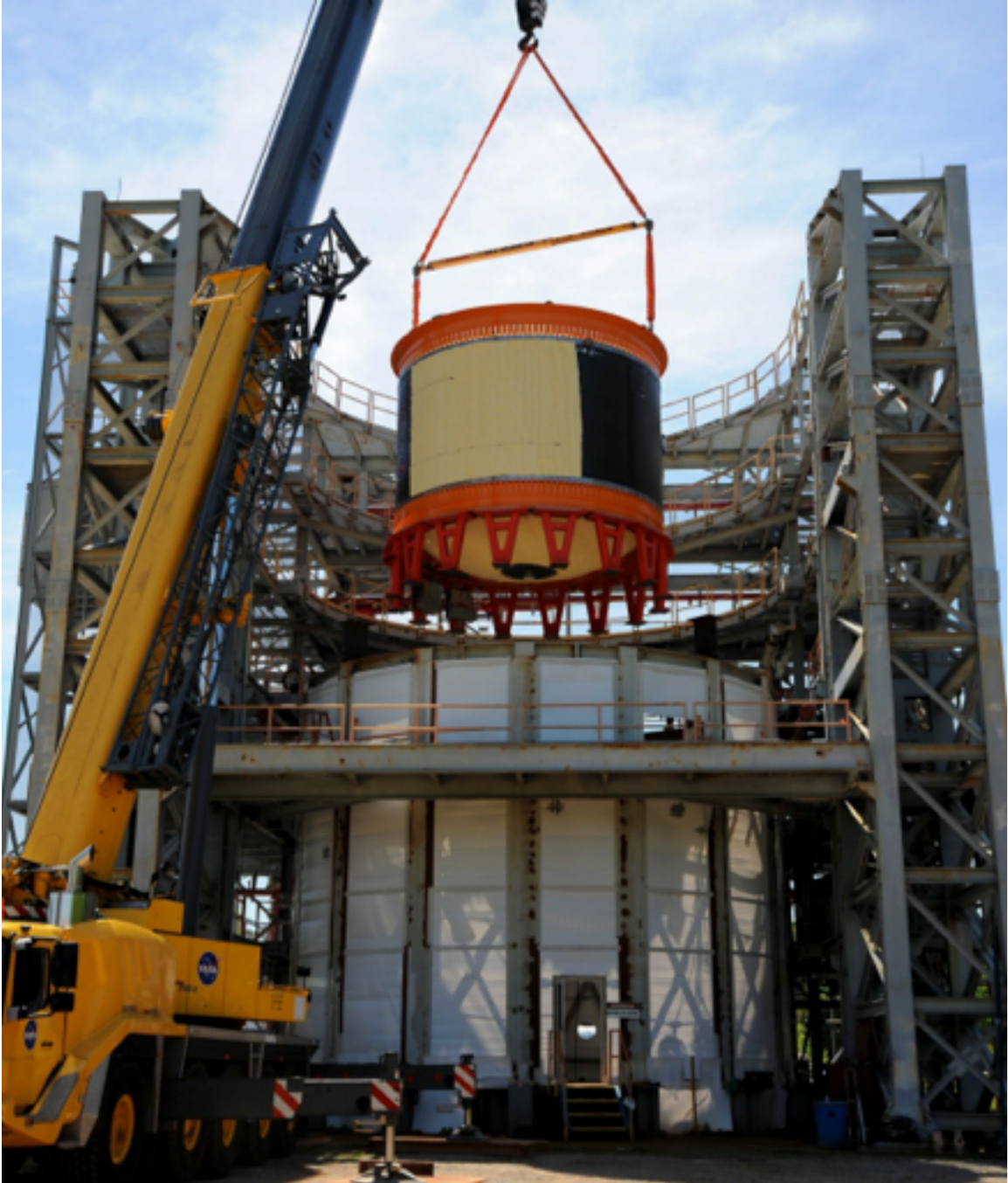
Figure 4. A ground test program was conducted for the 5.5-meter tank that included measurement of ambient pressure; cryogenic pressure; ambient pressure plus mechanical loads; and cryogenic cyclic pressure. Eighty-three pressure cycles were executed.
