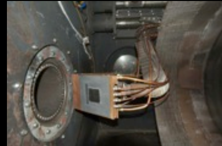
Carbon fabric arcjet testing (2012)
