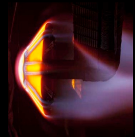
SPRITE C System level Arc-jet testing
