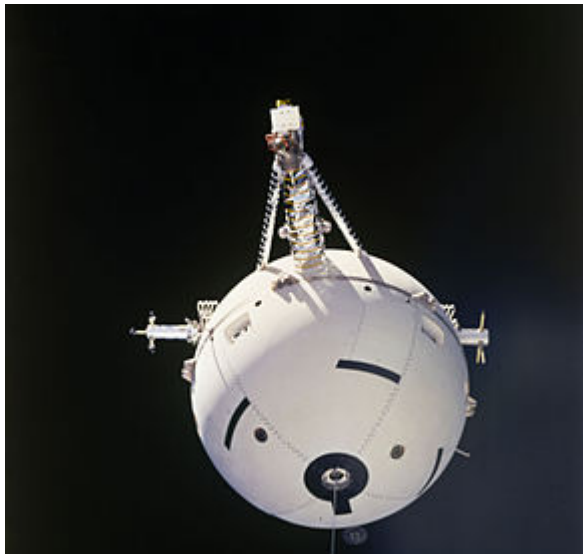
Figure 3 Close up view of TSS-1 from Space Shuttle Atlantis bay
