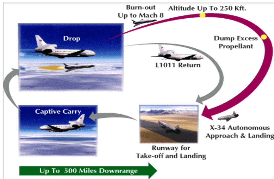
Figure 3 X-34 Flight profile ( http://www.allstar.fiu.edu/prime-tech/flight_profile.htm )
