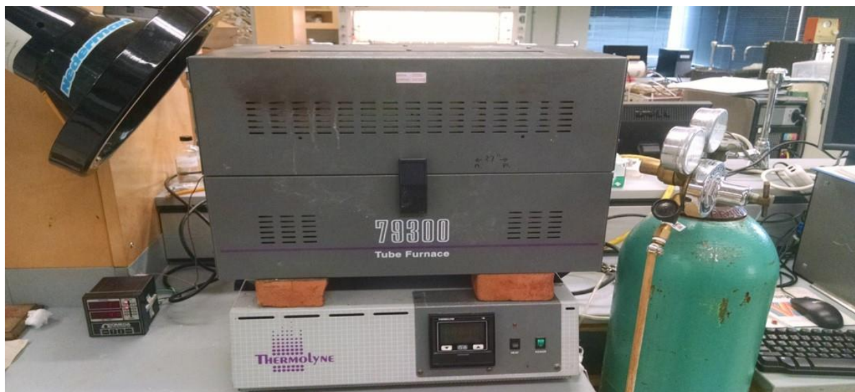
Figure 3. Horizontal furnace used for \text{Tl}_3\text{AsSe}_3 nanowire growth. This furnace suitable for melt and vapor transport growth of selenide materials
