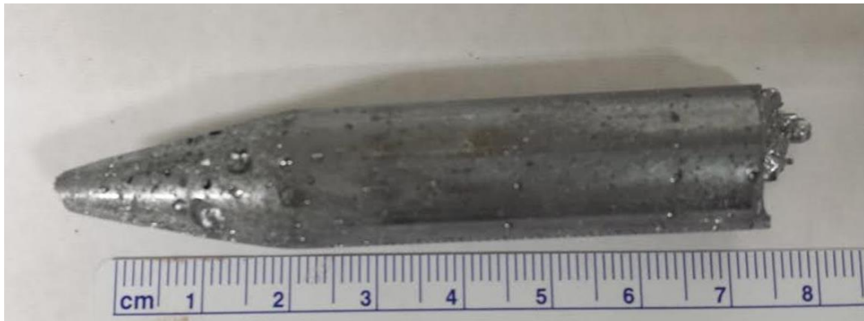
Figure 6- As-grown Tl 3 AsSe 3 crystal
