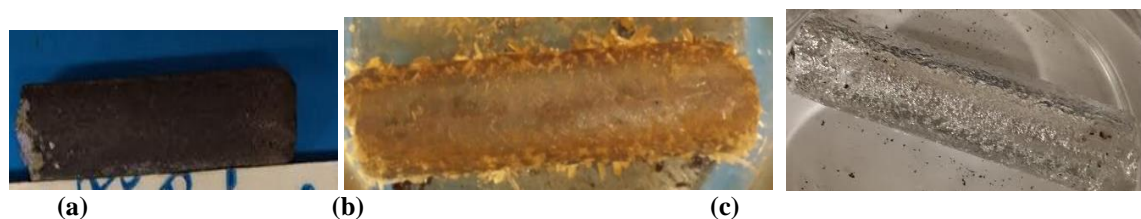
Figure 1. The (a) as supplied, (b) surface oxidized and (c) purified thallium is shown in the figure. Large whiskers of thallium oxide were observed when thallium was placed in dilute acid.
