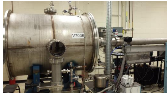
Figure 4. Side view of target chamber showing pumping system.
