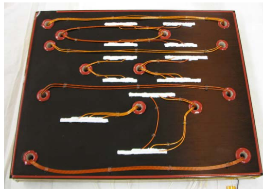
Figure 3. Front Side Wire Coupon. The coupon represents wiring used to connect sections of the solar array together. Wire pairs are typically configured with a power system positive lead next to a return (or ground) lead.
