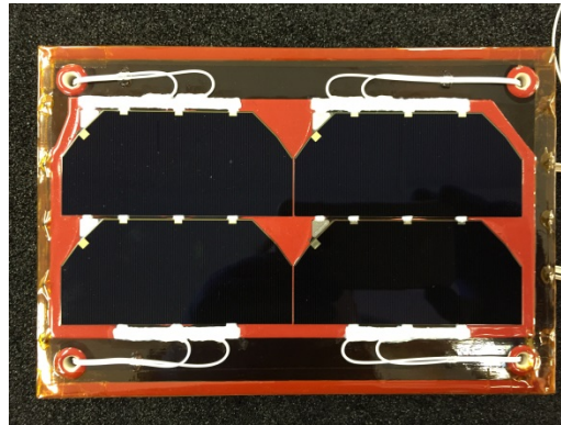
Figure 2. Cell-Interconnect-Coverglass (CIC) coupon. The coupon is composed of 2 strings. Each string is formed by connecting 2 cells in series.
