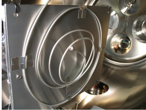
Figure 6. Coaxial cable sample. The cable is a semi-rigid cable with an Aluminum outer jacket. Each end of the cable is terminated with SMA male connectors. The sample was formed into a spiral geometry to maximize the area of the cable exposed to the electron beam.
