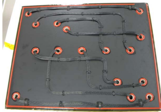
Figure 4. Back Side Wire Coupon. This coupon represents the wiring on the back side of a solar array. The backside of the solar array employs a conductive Kapton material (which is black in color). Like the front side coupon, pairs of wires can represent the positive and return wires associated with the power system.
