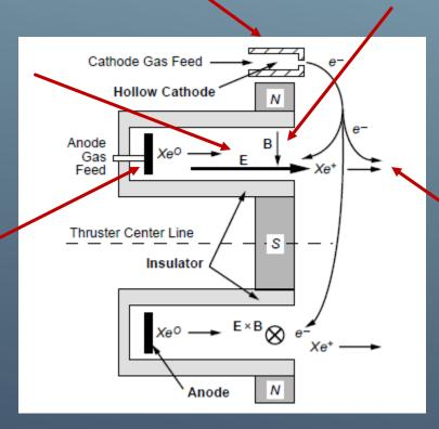
Radial B field prevents electrons from streaming directly to the anode, instead spiraling along the B field lines in the E x B azimuthal direction (Hall Current) and diffuse to the anode ionizing the propellant.
