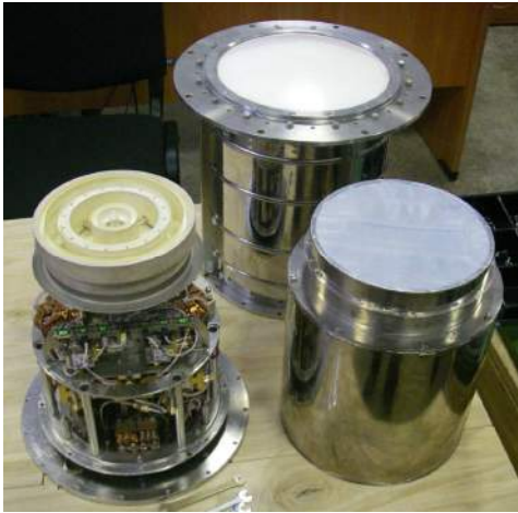
Fig. 2 Cryostat assembly: equipment, container with vacuum window, thermal screen.
