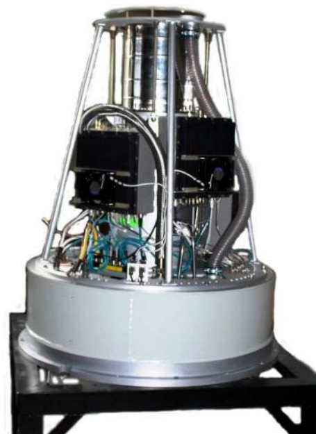
Fig. 1 Tri-band receiver focal container (without housing).
