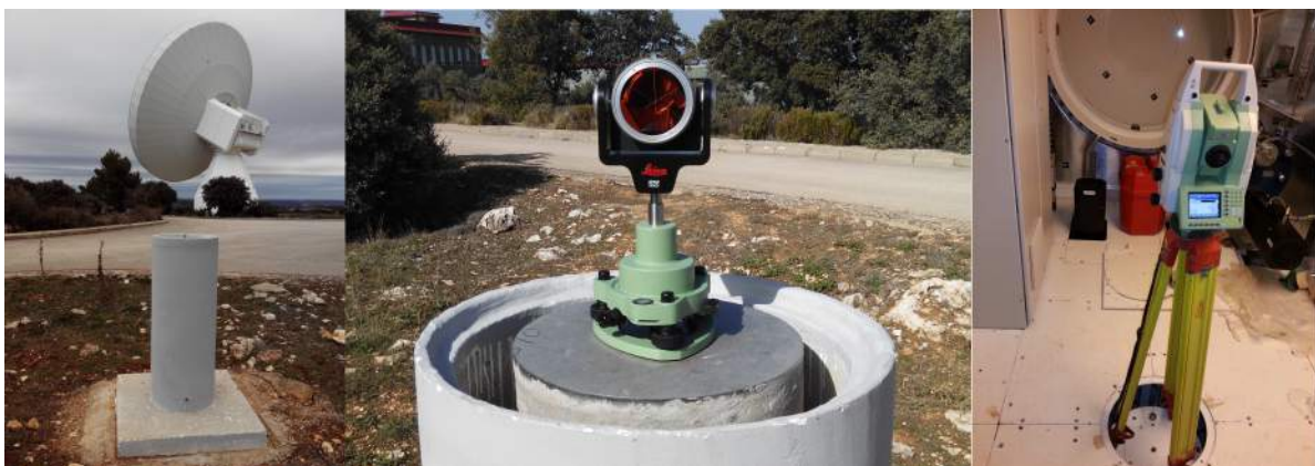
Fig. 3 Left: Vertex monument in Yebes. Middle: Reflector RRR attached magnetically to the inner side of one counterweight. Right: Robotic Total Station Leica TS-30 set up above the central pillar.
