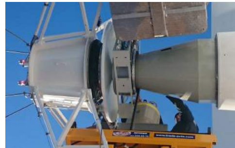
Fig. 4 Telescope receiver calibration with load.
