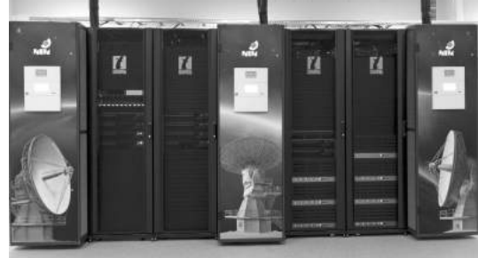
Fig. 2 View of the high-performance computing cluster based on the hybrid blade servers.
