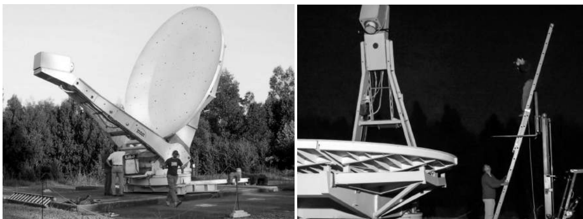
Fig. 3 (Left) The VLBI telescope primary mirror covered with reflecting targets for photogrammetry measurements. (Right) Pictures taken at different angles with the telescope pointing at 110 degrees of elevation. Credits: Rolando Dünner/AIUC.
