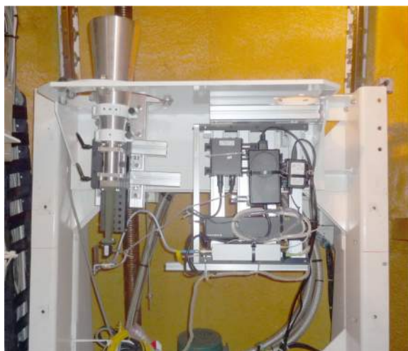
Fig. 2 Broadband (IGUANA) feed installed in the receiver room of the Kashima 34-m telescope.
