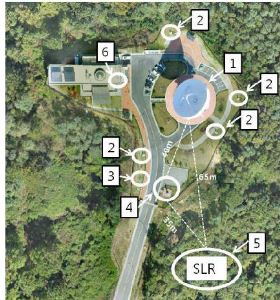
Fig. 1 Layout of Sejong station: 1. VLBI antenna 2. pillar for co-location 3. UTP(Unified control Point) 4. IGS station (SEJN) 5. (Under construction) SLR site of KASI 6. (Under installation) MR(Microwave Radiometer) of KASI.
