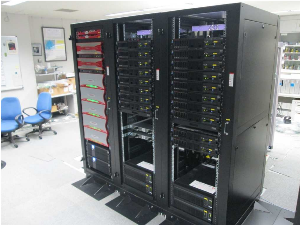
Fig. 1 View of the data processing servers and storage system at the Tsukuba VLBI Correlator.
