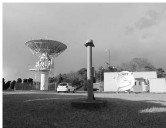
Fig. 4 GNSS receiver pillar at the Kashima 11-m site registered as KSMV of the IGS tracking station.
