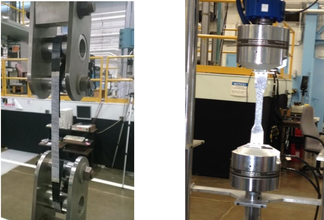
Figure 5. Strap (constant width) specimen in Mil-T-87130 double-pin grip fixture (left) and dogbone specimen in hydraulic grip fixture (right) installed in universal testing machine for tension tests.
