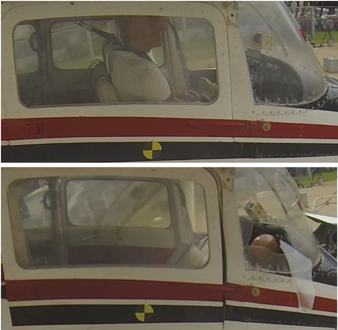
Figure 17 - Test 2 co-pilot head flail. Before impact (top) and max flail (bottom)
