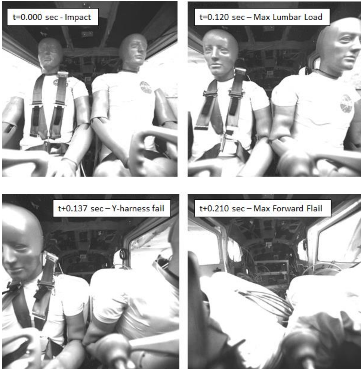
Figure 15 - Test 2 occupant motion sequence - onboard camera
