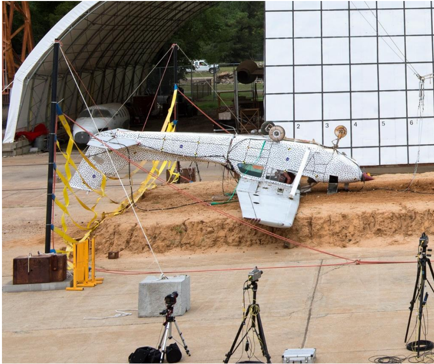
Figure 26 - Post-test orientation of airplane in Test 3
