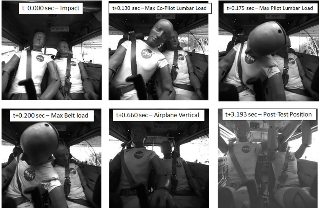
Figure 28 - Test 3 occupant motion sequence - onboard camera
