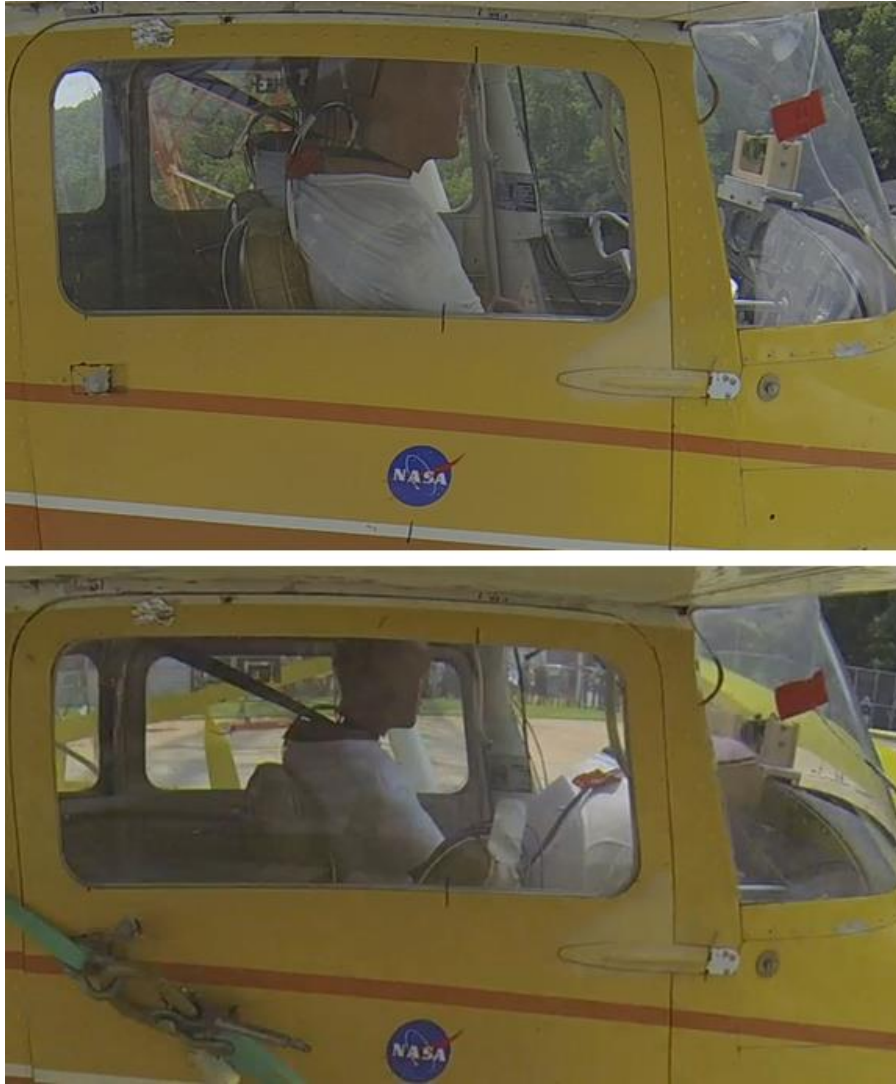
Figure 7 - Test 1 co-pilot head flail. Before impact (top) and at max flail (bottom)
