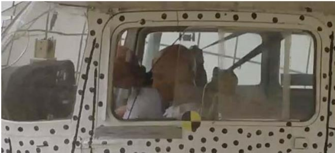
Figure 29 - Test 3 pilot head flail. Before impact (top) and max flail (bottom)
