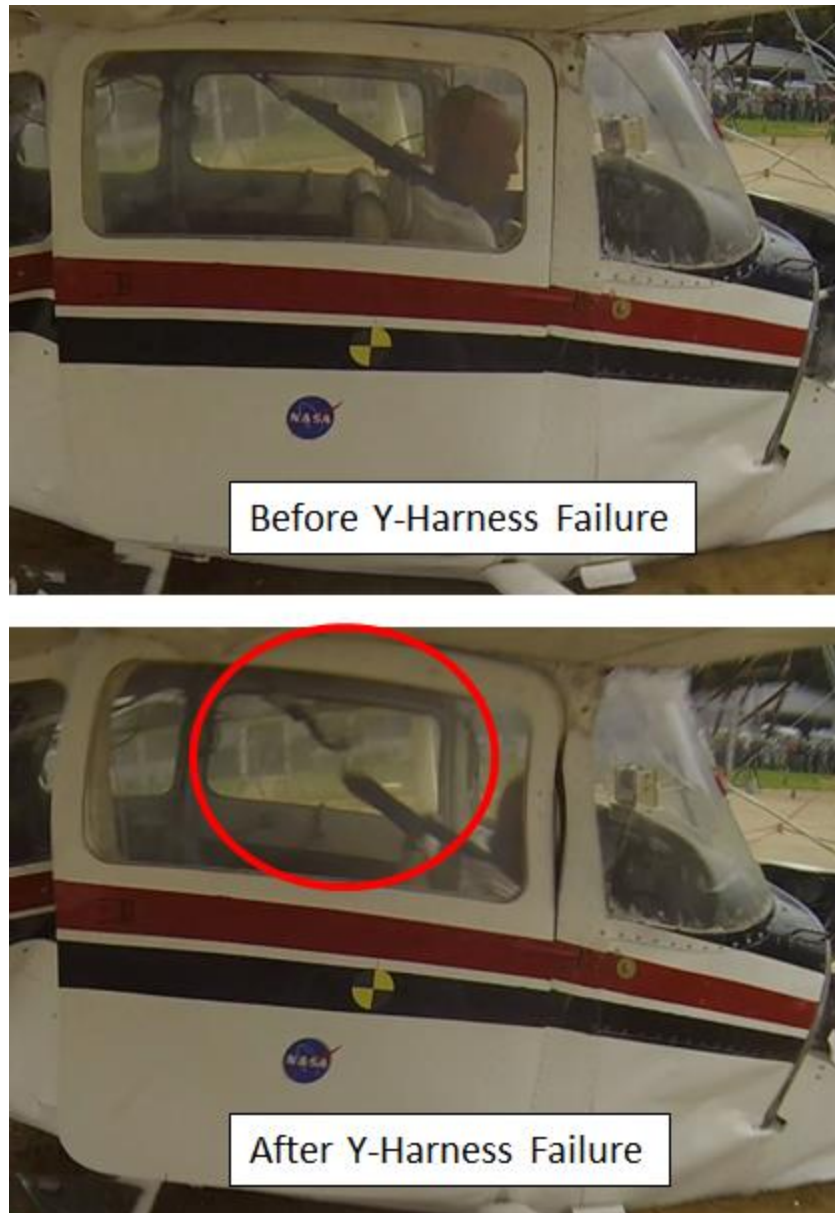
Figure 18 - Test 2 y-harness failure
