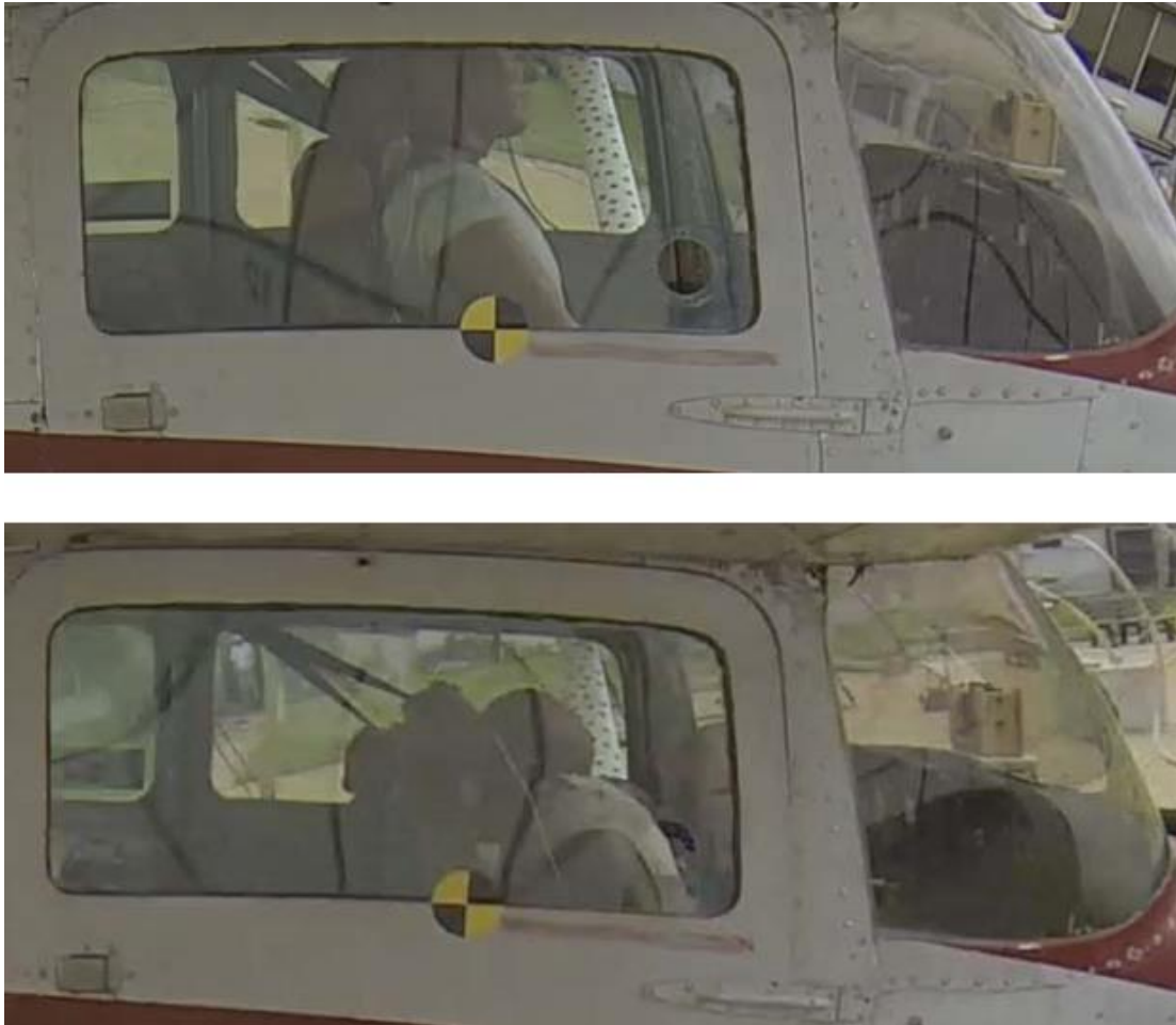
Figure 30 - Test 3 co-pilot head flail. Before impact (top) and max flail (bottom)
