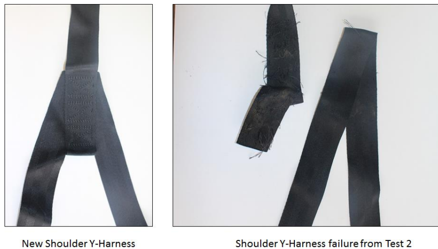
Figure 20 - Test 2 shoulder y-harness failure
