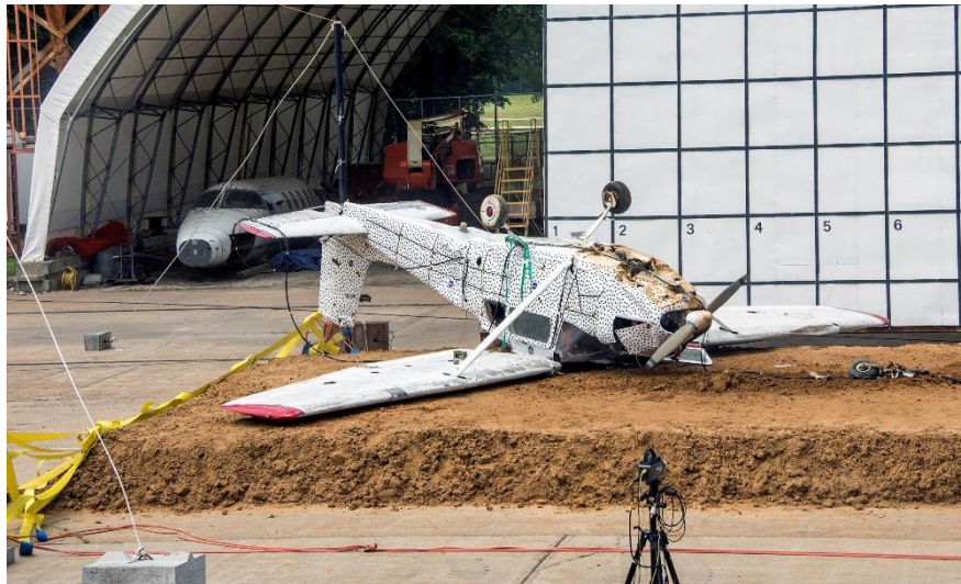
Figure 12 - Post-test orientation of airplane in Test 2
