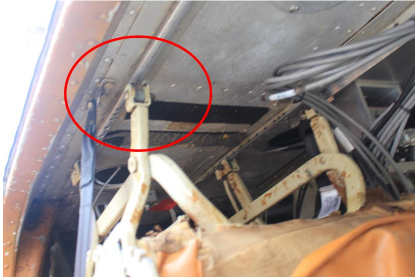
Figure 35 - Test 3 co-pilot seat pullout
