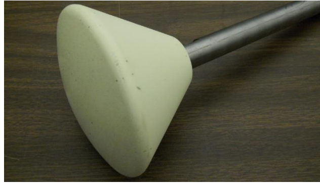
Fig. 6: A CEV blunt body model used for BOS testing in the 31-Inch Mach 10 Air Tunnel in September, 2012.
