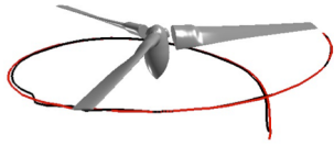
Figure 9: Vortex core lines generated by using the local maximum Q_s (black curve) and the local minimum pressure (red curve) using dataset #2 (medium grid resolution).
