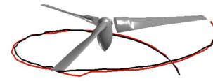
Figure 7: Vortex core lines generated using the local maximum Q_s (black curve) and the local minimum pressure (red curve) using dataset #1 (coarse grid resolution).
