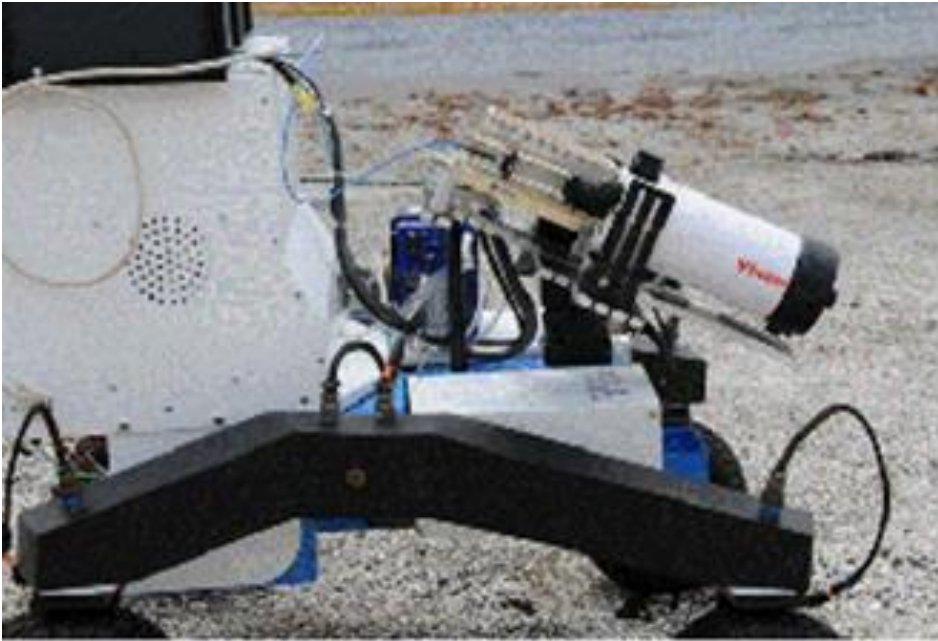
Figure 5. Remote Raman, Fluorescence, and Lidar Multi-spectral Instrument.
