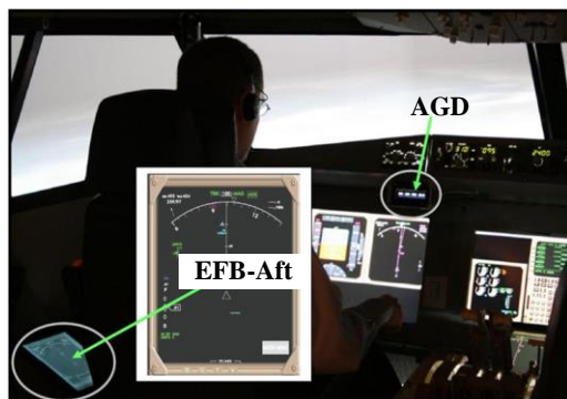
Figure 1. The Integration Flightdeck Simulator, showing the EFB in the Aft position, and the AGD.
