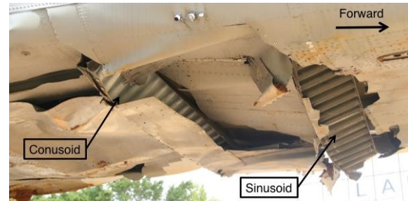
Figure 21. Post-test photograph of outer skin deformation between FS220 and FS286
