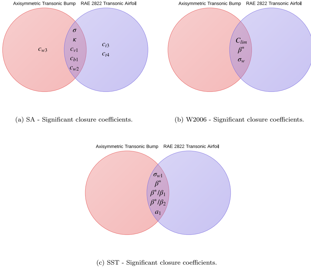
Figure 10. Closure coefficients significant to uncertainty in at least one output quantity of interest for each CFD problem and for each turbulence model.
