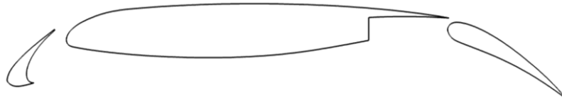
Figure 2. Cross-sectional view of the 3-element 30P30N high-lift configuration.
