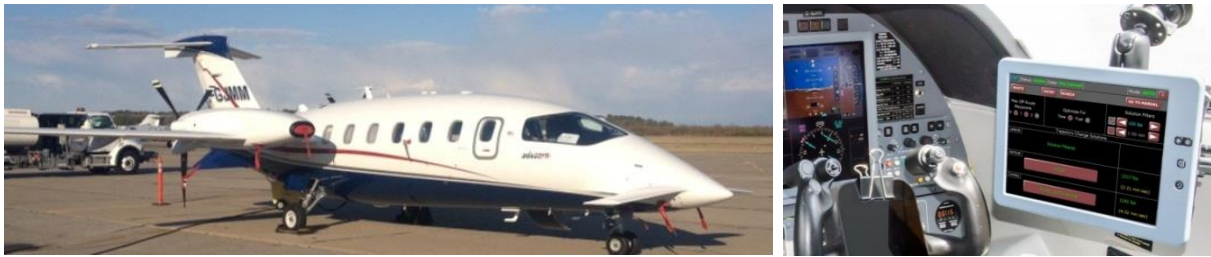
Figure 5 Piaggio Avanti flight test aircraft with TAP (and its earlier HMI) installed on a United Technologies Corporation (UTC) G500 SmartDisplay™ EFB.
