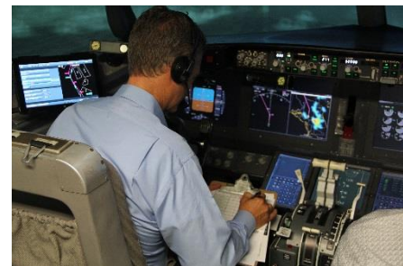
Figure 4 Operator Performance Lab simulation cab showing the TAP application to the pilot's left. Photo by M. Cover.
