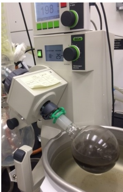
Figure 6: Acetone Evaporating from a Spiked Lunar Simulant Using a Rotavapor
