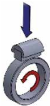
Figure 4. Schematic of block-on-ring test.
