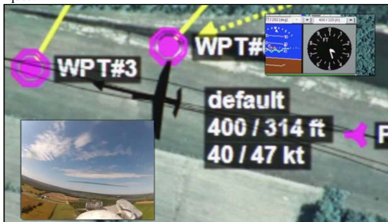
Figure 2: Automatic Go-Around Initiated at 200' AGL Due to Glide Slope Error
