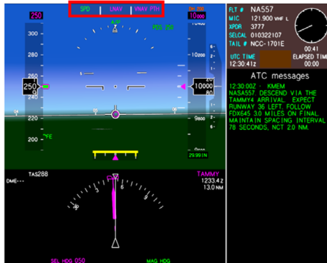
Figure 11. Identification of FMA on PFD.
