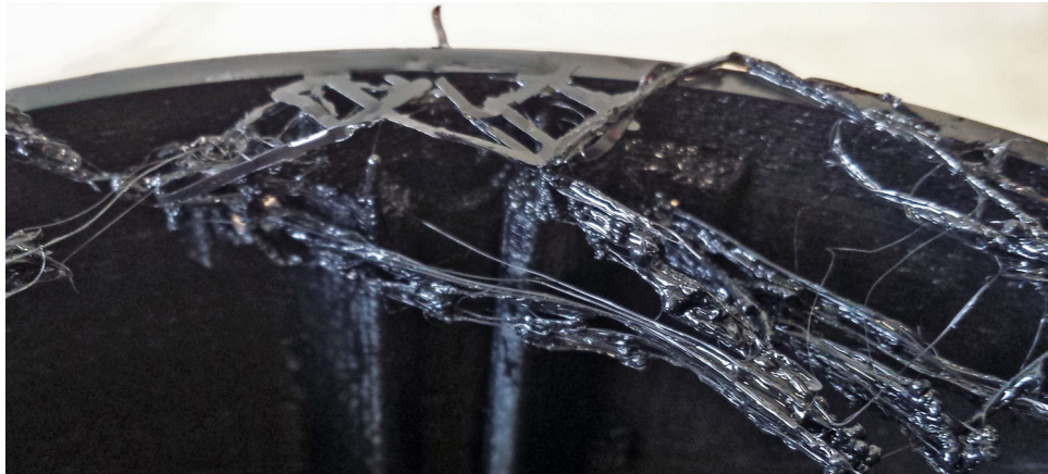
Figure 4.9: Residue given by non-retracting filament in Cube Module print.
