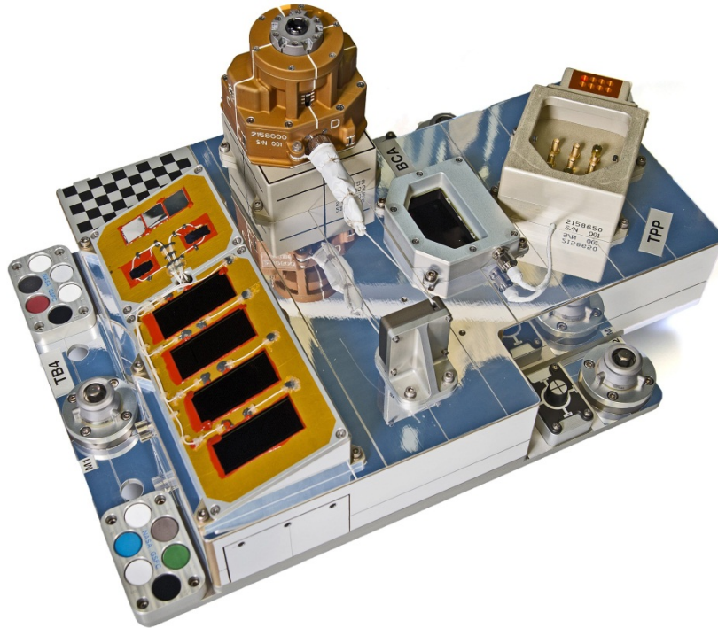
Figure 5. Fully integrated TB4 showing SCE passive samples (GSFC).
