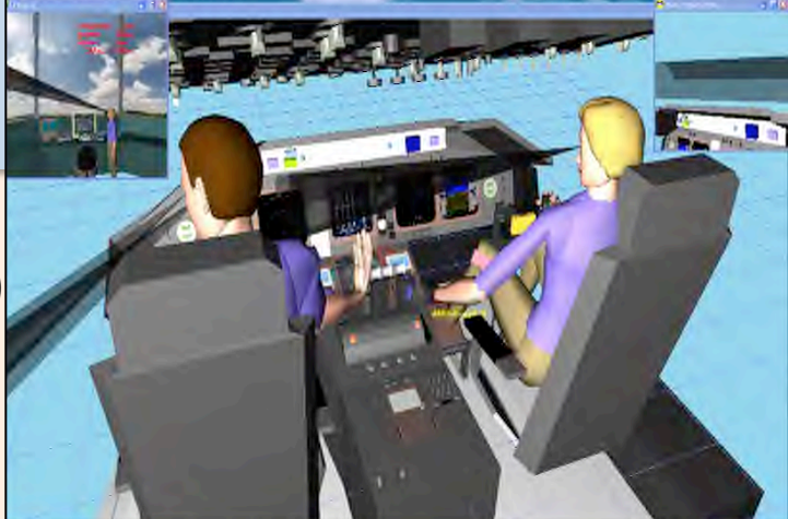
MIDAS v5, a human performance model of the flight deck environment, pilots' workflow and cognitive processes.
