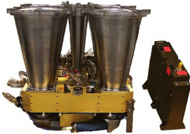
Figure 1. Photograph of MLA at GSFC prior to delivery to MESSENGER. The diameter of each of the four receiver telescopes is 14 cm.
