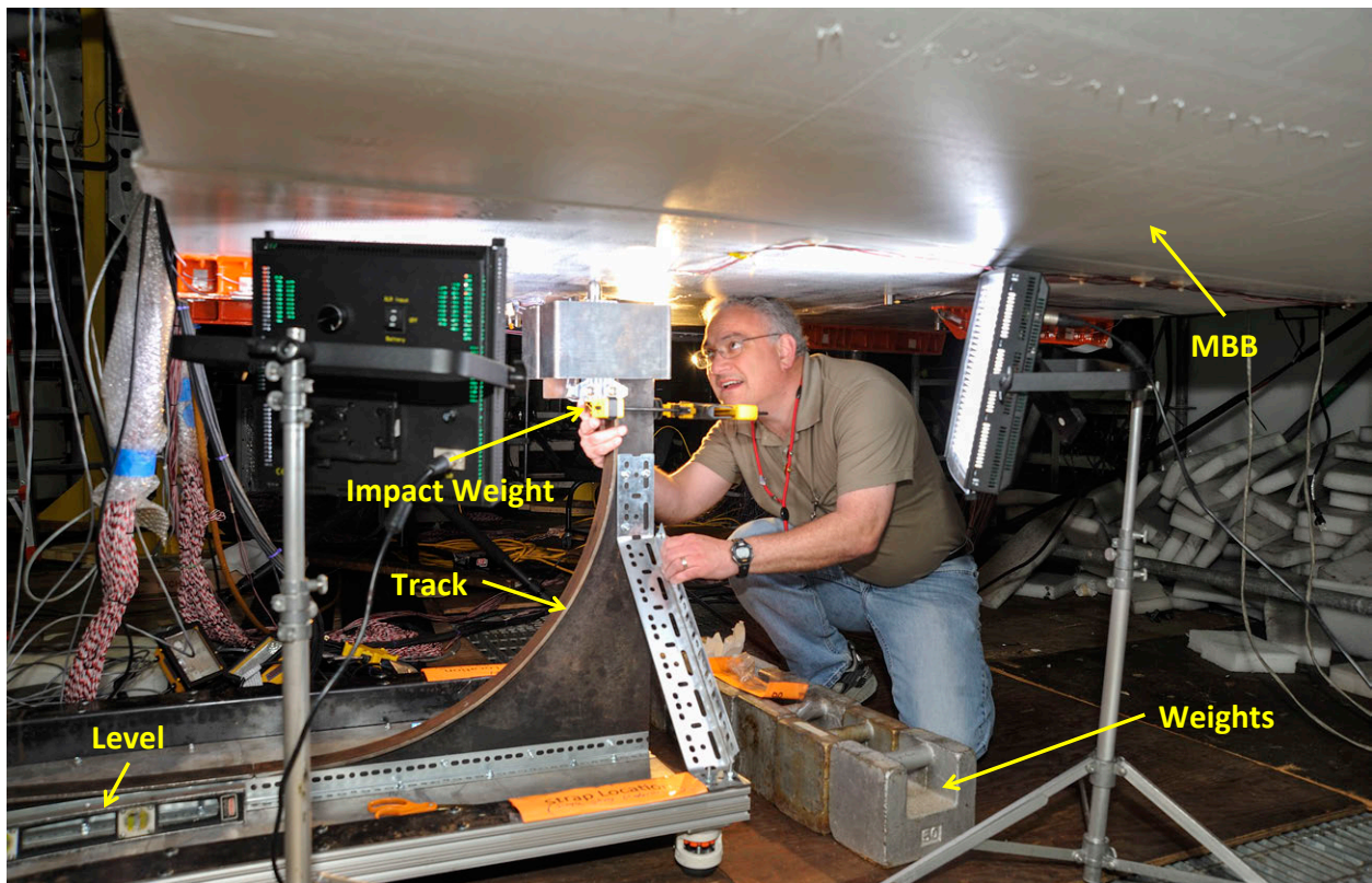
Figure 15. Alignment of impactor for exterior skin impact.
