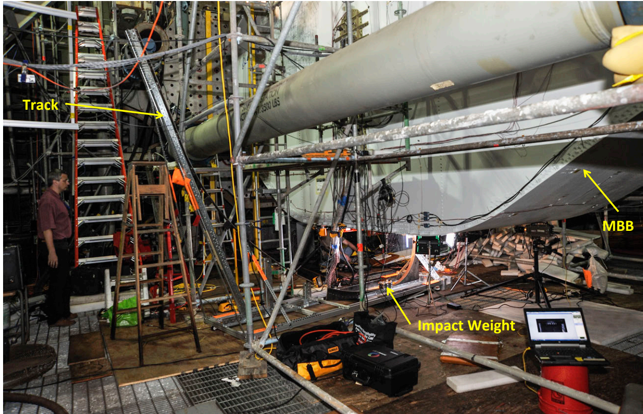
Figure 14. Impactor in COLTS in location to impart exterior skin BVID to MBB keel.
