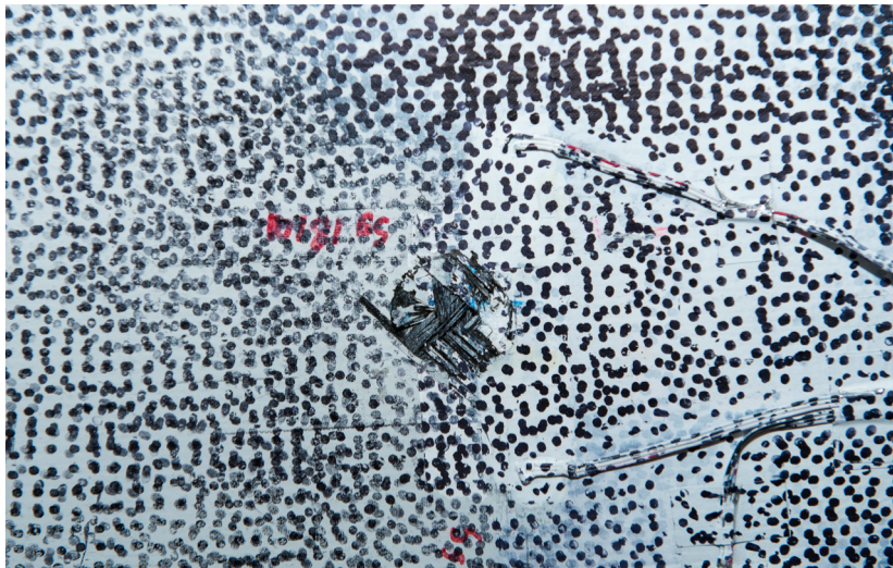
Figure 19. Impact causing a through-hole.
