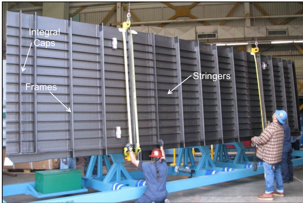
Figure 3. PRSEUS panel being prepared for assembly.
