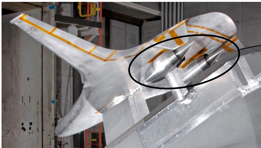
Figure 12. BENS engine nacelles in inlet and exhaust noise radiation configurations (nacelles shown in their nominal position with respect to the model airframe).
