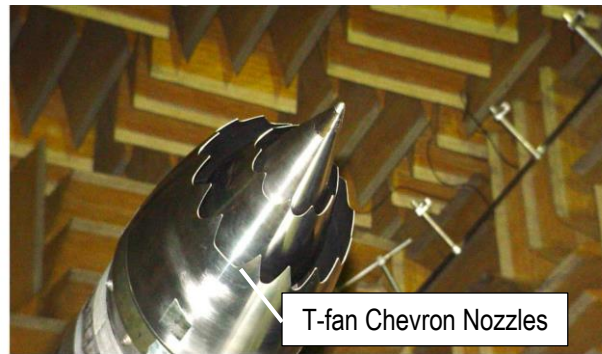
Figure 15. "F8" low-noise chevron nozzle in NASA Langley's Low Speed Aeroacoustic Wind Tunnel.
