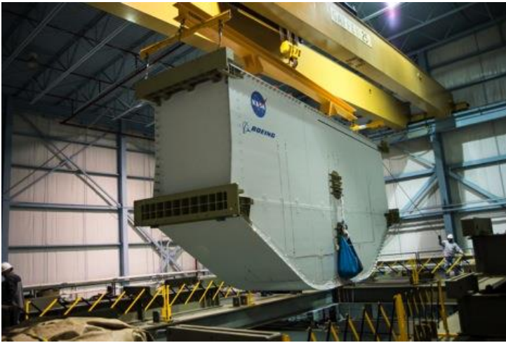
a Multi-bay pressure box suspended from crane above test chamber
