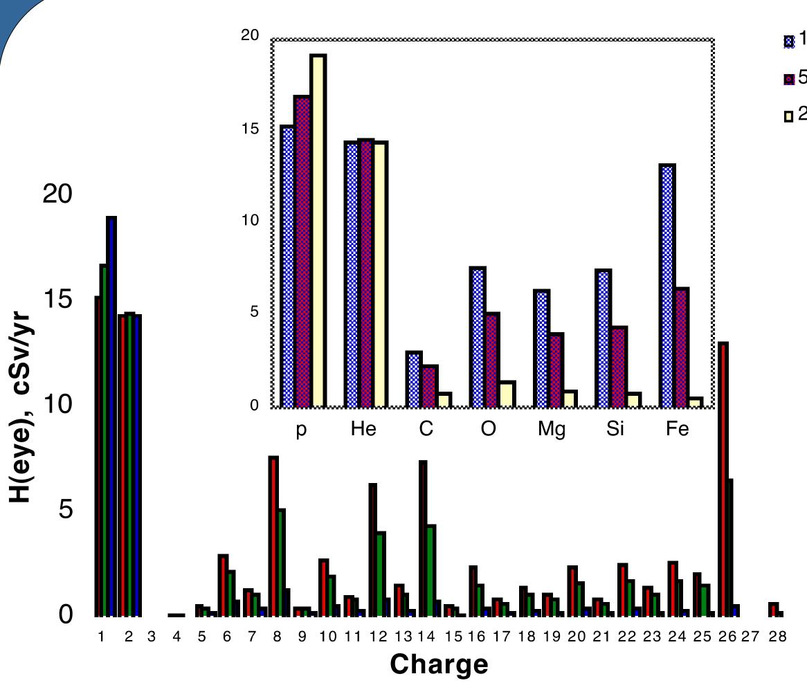
Average dose equivalent rate (H) from exposure of the eye behind various thicknesses (1, 5, 20 g/cm<sup>2</sup>) of polyethylene slab shielding at solar minimum. Red, green and blue bars in the lower portion of the figure represent 1, 5 and 20 g/cm<sup>2</sup> respectively. The most significant components are shown in the inset. Reprinted from [Schimmerling et al., 1999].
