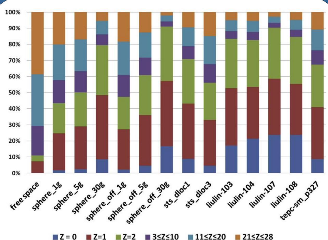
Calculations of percent contribution to blood forming organ (BFO) dose equivalent by charge group for free space (far left), simple spherical geometries in free space, and various detector locations inside the space shuttle (STS) and the International Space Station (ISS) in free space. This figure does not show data, but only calculations at detector locations. Reprinted from [Walker, Townsend & Norbury, 2013].
