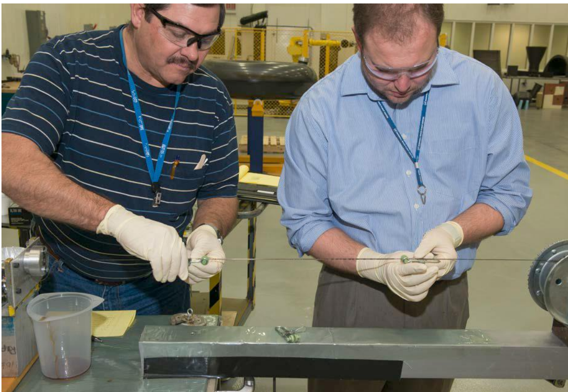
Figure 5.3-3. Fabrication of Carbon Strands for Stress Rupture Failure Testing. A winch (right) is used to draw the carbon fiber material through the die (left). Phil Thompson (L) and Chad Hastings (R) demonstrate a preparation step before the test article is cut to length.
