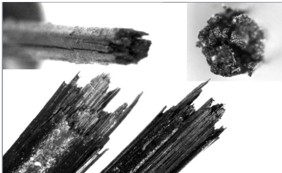
Figure 6.2-5. Fractured Ends of SN 8407 Showing Multiple Axial Splits
