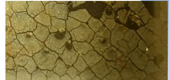
Credit: NASA/Langley/Elaine Seasley Molecular Contamination Film
