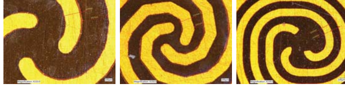
Figure 9: Photo-lithography method used in copper on polyimide film panels of increasing electrode densities
