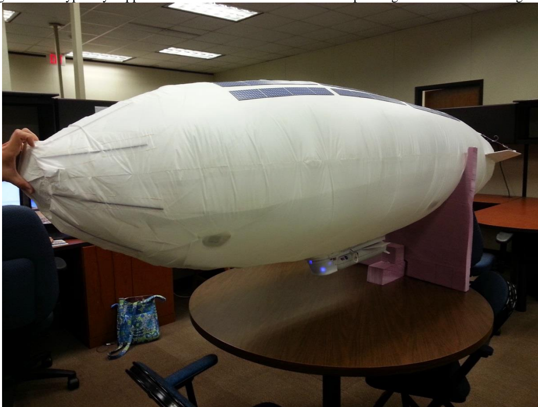
Figure 9: Inflated airship model with gondola containing habitat and ascent vehicle.
