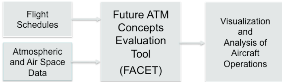
Figure 1. Global air traffic simulation using FACET and analysis tools.
