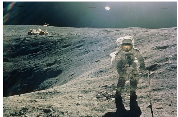
Fig. 14. Astronaut Charlie Duke during Apollo 16 using a bore hole tool for vertical profile samples of the lunar regolith.
