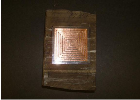
Fig. 7. Proof-of-Concept Sensor on geologic core sample.
