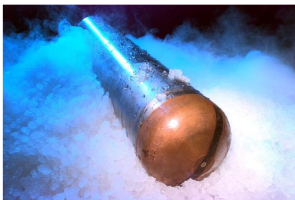
Fig. 11. Cylindrical thermal melt probe penetrator.
