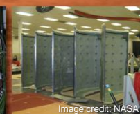
Water Filled Composite Shield Sections
