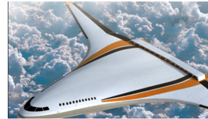
boundary-layer ingestion for drag reduction
