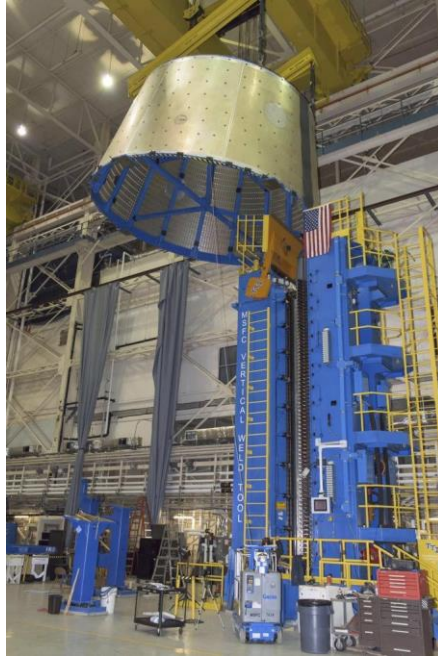
Figure. IX: Aft cone of LVSA test article moves out of weld tool at MSFC.
