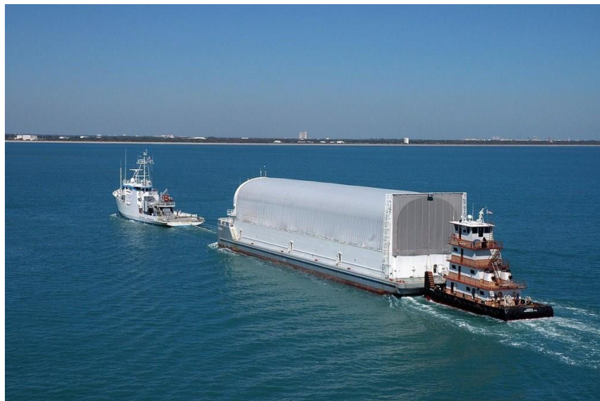
Figure. XI: Lengthened Pegasus barge delivered to SSC to support SLS core stage testing and transportation.
