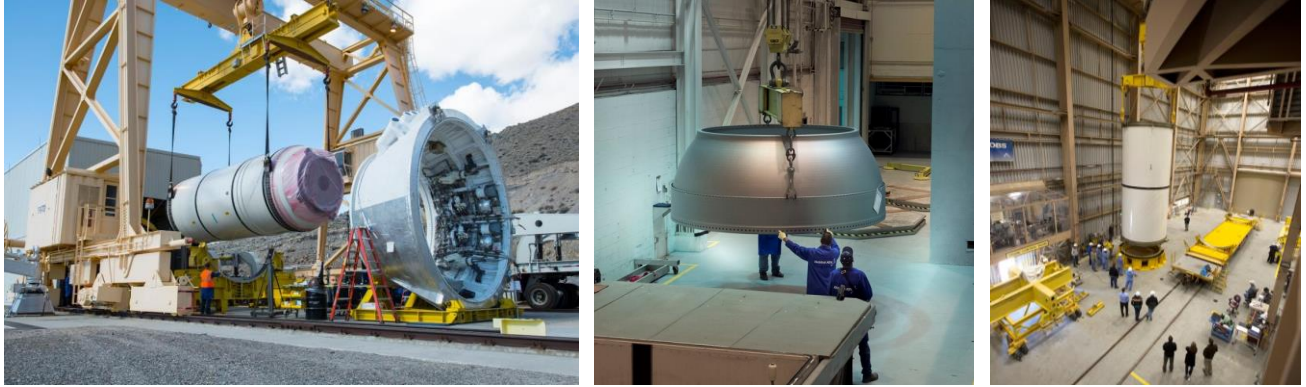
Figure. VIII: Fifth segment for QM-2 delivered to test site (left), aft dome for EM-1 booster (center), booster pathfinder hardware at KSC.
