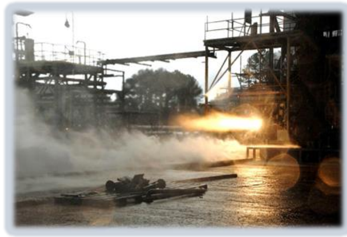
Figure 4: Sub-scale injector hot fire test
