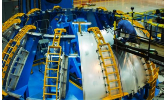
Figure 3. A technician inspects a core stage dome weld on the Gore Weld Tool at MAF, July 2015.
