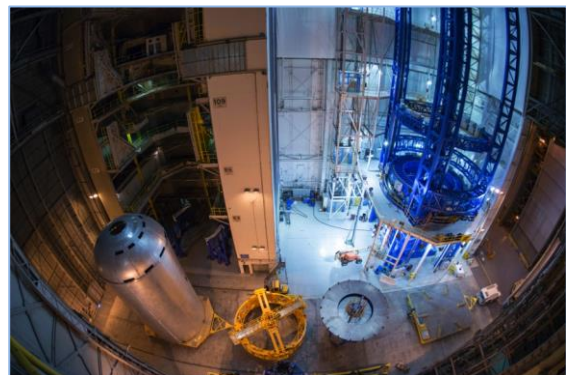
Figure 4. SLS core stage liquid hydrogen tank weld confidence article, left, completed Welding on Vertical Assembly Center, February 2016, at Michoud Assembly Facility.
