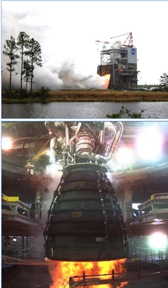
Figure 6. Top, EM-2 flight engine 2059 test fired at Stennis Space Center. Bottom, close-up showing engine operation.
