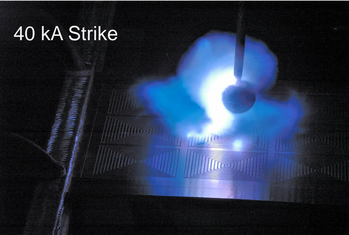
Test Strike on Panel
