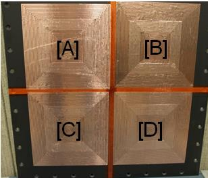
8 inch SansEC Array (before paint)
